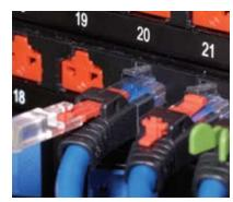
To prevent accidental disconnects, but still give people access to ports, use the green Secure Lock cable. The Secure Lock holds the cable in place and eliminates accidental disconnects from jostling and general wear and tear. To release the lock, just squeeze the butterfly tabs.
