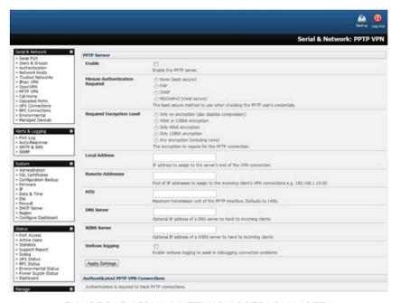
FIGURE 5-35. SERIAL & NETWORK: PPTP VPN SCREEN
