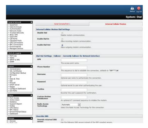
FIGURE 6-3.SET UP DIAL-OUT PPP CONNECTION SCREEN
