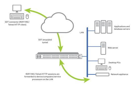
FIGURE 4-15. SDT CONNECTOR APPLICATION EXAMPLE
