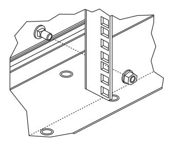
Figure 1-3. Adjusting the rails.
