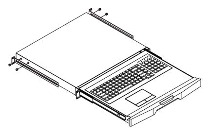
FIGURE 1. INSTALLING THE FASTENERS ON THE RM419-R5
