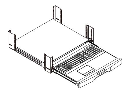
FIGURE 3. INSTALLING THE RM419-R5 KEYBOARD DRAWER INTO THE RACK
